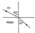
Angle of incidence, i = 60° Angle of refraction, r = 47° According to Snell's law,
