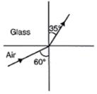
Angle of incidence, i = 60° Angle of refraction, r = 35° According to Snell's law,
